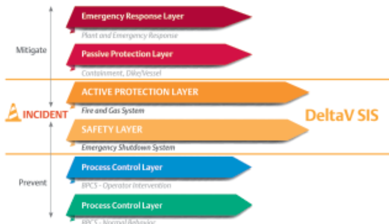
FIGURE 1. Providers of automation and safety systems suggest looking at “layers of protection” to ensure the highest level of safety
