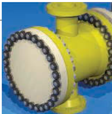
FIGURE 2. A hydraulic nut on a heat-exchanger flange helps to maintain proper tightness, since the nut stays in place even after a breakout
