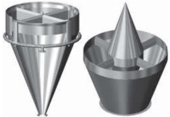
FIGURE 9. Improved gas uniformity can be achieved by injecting gas via crossbeams and an annulus, such as those shown here
