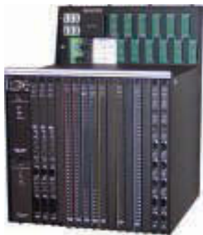
FIGURE 4. Schneider Electric provides safety protection via the Triconex safety instrumented system, which controls emergency shutdown to help prevent disasters
