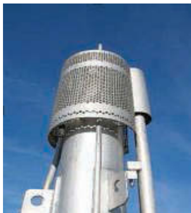
FIGURE 5. A typical flare burner tip helps to dissipate hydrocarbon gases via combustion, and can be located at ground level or on an elevated structure
