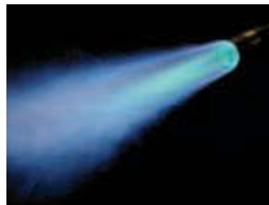
FIGURE 3. Pilot burners use electrical current to detect the flame's presence
