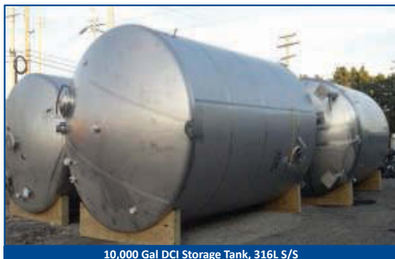
10,000 Gal DCI Storage Tank, 316L S/S
